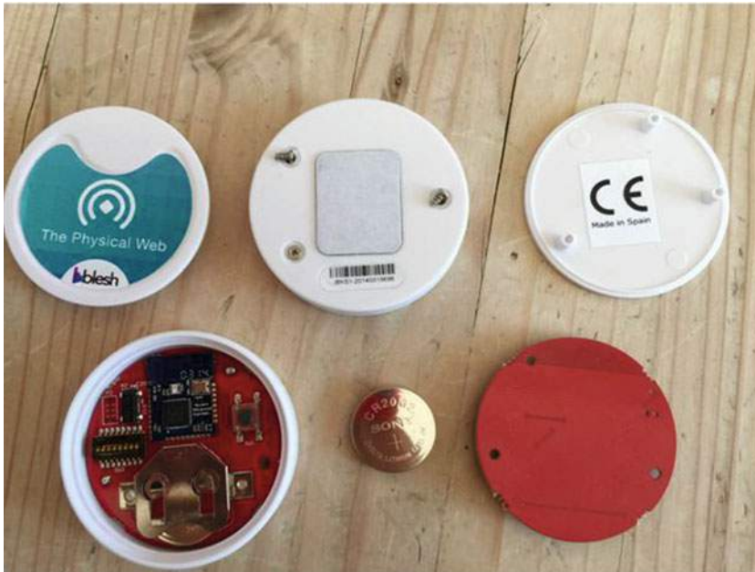
Figure 5-28. Inside a Blesh Physical Web beacon
