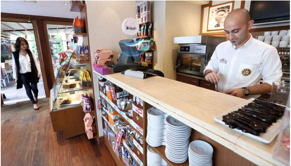
Figure 21-7. Customers enter the café with their phones in their purse and the phone detects the Blesh beacon and sends the customer’s details to the iPad on the counter of the café without any intervention by the customers
