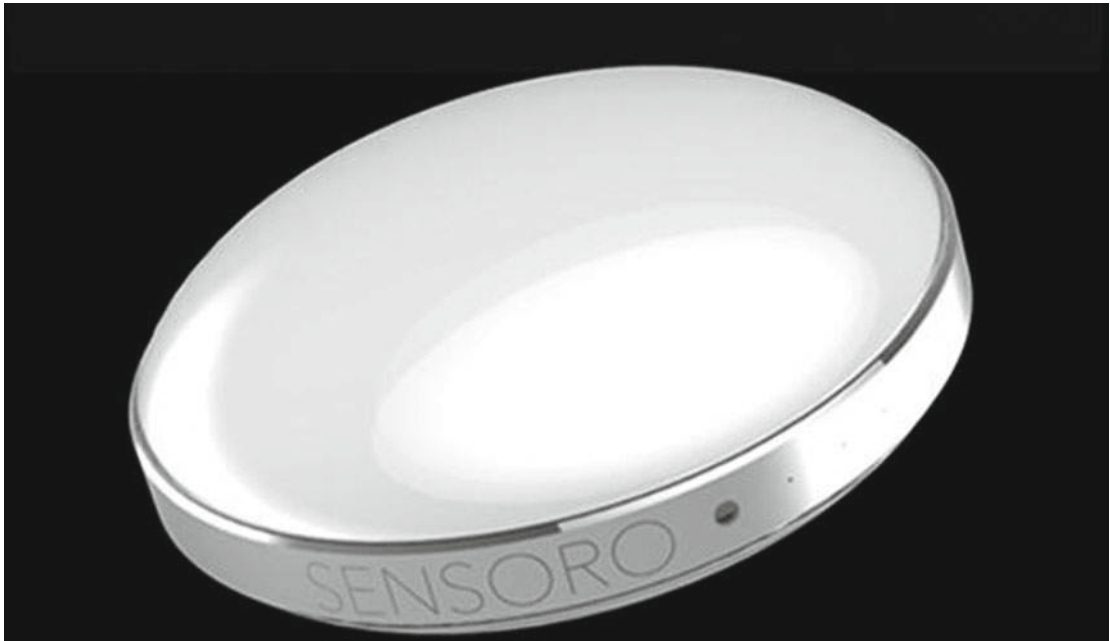
Figure 7-4. The Sensoro Yunzi beacon combines aesthetics with a more discrete package
