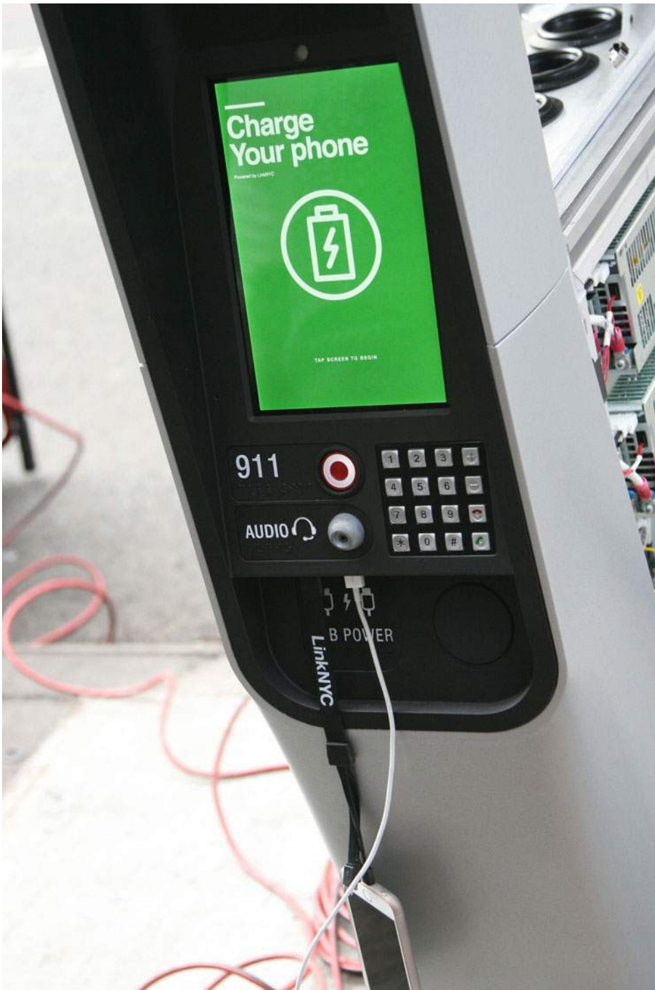
Figure 13-18. Link station being set up; the kiosks offer phone charging, Internet browsing, free phone calls, and emergency services calling
