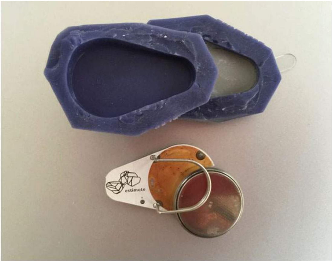
Figure 7-6. Inside an Estimote beacon, cut open to reveal the motherboard and battery
