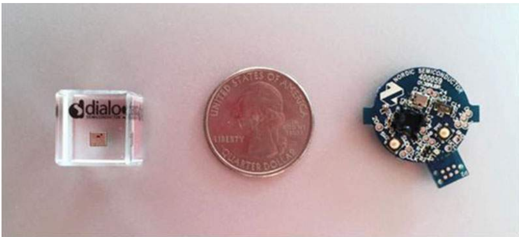
A Dialog Bluetooth Smart SoC and a Nordic Bluetooth Smart Module
