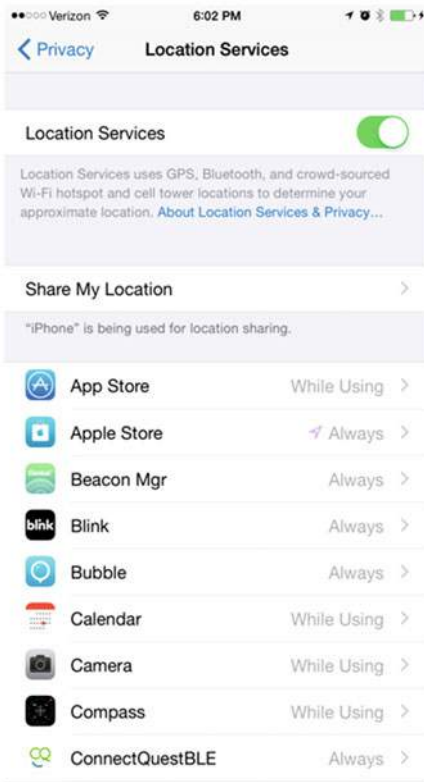
Figure 5-5. The panel in iOS settings that allows users to control privacy and the ability for an app to be triggered by an iBeacon
