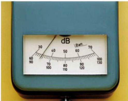
Figure 5-11. A meter measuring signal strength in dB
