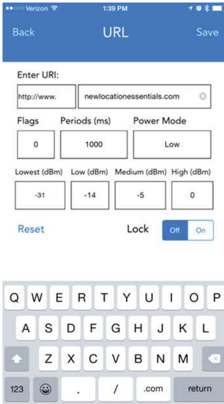
Figure 5-29. The Blesh app's Physical Web configuration screen allows the beacon's URL to be set
