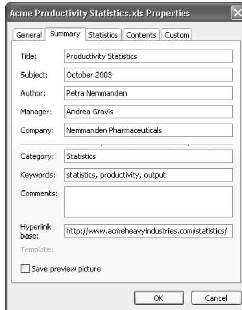
FIGURE 3-2 You can enter key information on the Summary tab of the Properties dialog box to make workbooks easier to identify without opening them.
