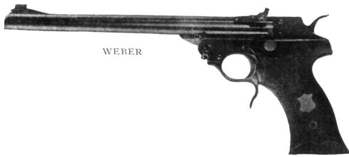
Fig. 16—ADOLPH WEBER PISTOL Ten-inch barrel; weight, 2 lbs., 2 oz.; .22 cal.
