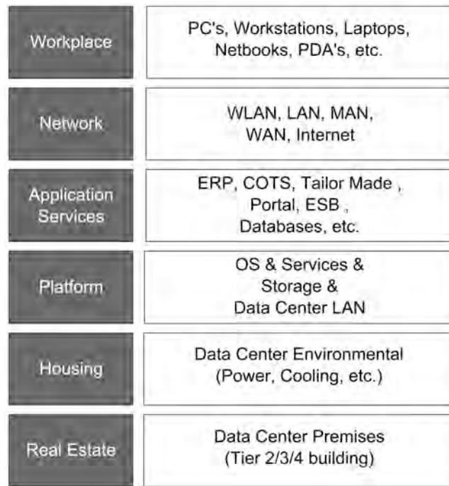
Figure 4.2: An example of an IT service stack
